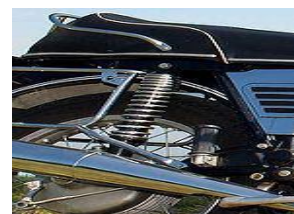
Fig 1.1:- Rear shock absorber and spring of a BMW R75/5 motorcycle
